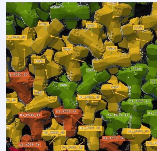
Visualisation of movements within the embankment, block by block
